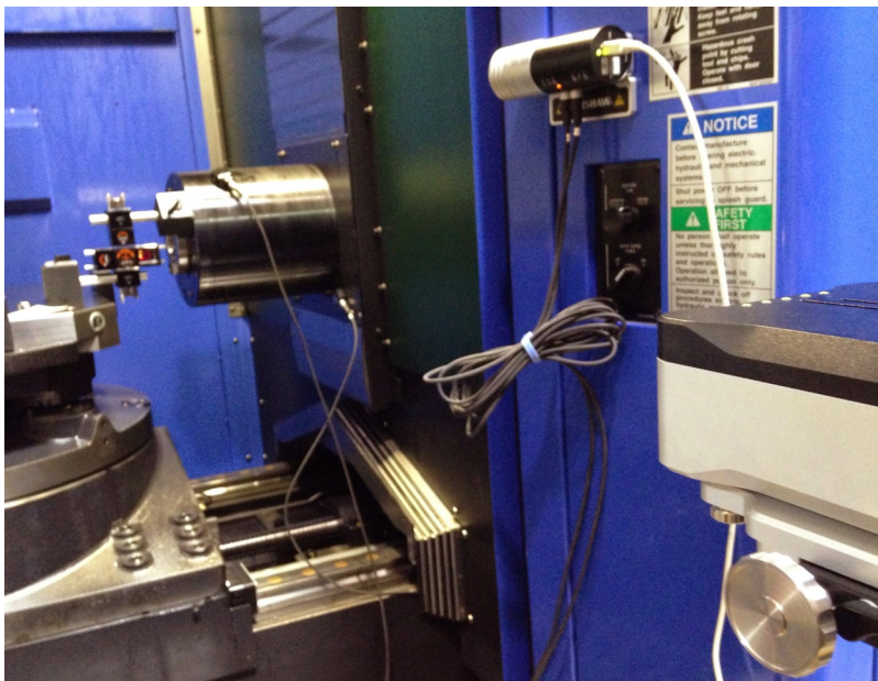
Renishaw XL-80 Interferometer on a small horizontal Mill
